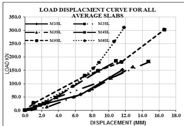
Figure 5. Load-displacement relations for all slab types
