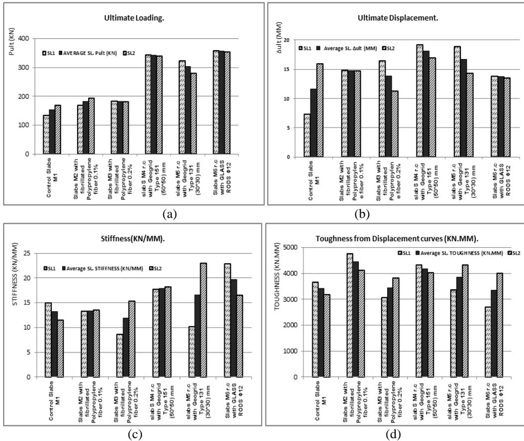
Figure 4. Effect of different reinforcement types on (a) ultimate load, (b) maximum displacement, (c) stiffness and (d) toughness
