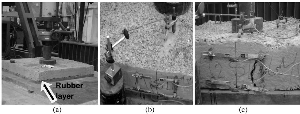
Figure 3. Testing and instrumentation: (a) test setup, (b) LVDT and (c) strain bi-gauge
